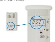
The code number on the test strip container and the test strip code chip must match.
