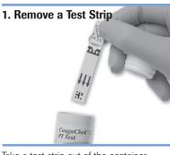
Take a test strip out of the container. Close the container tightly.
