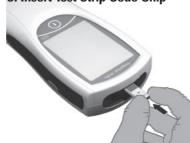
With the code number facing up, insert the code chip into the code chip slot until it snaps into place.
