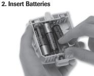
Insert 4 AA batteries according to the diagram inside the battery cover. Replace the cover.
